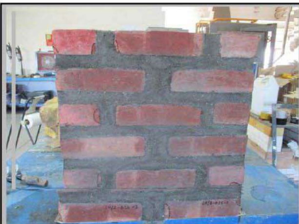
Photograph 1: Image of the panel before freeze/thaw cycles
